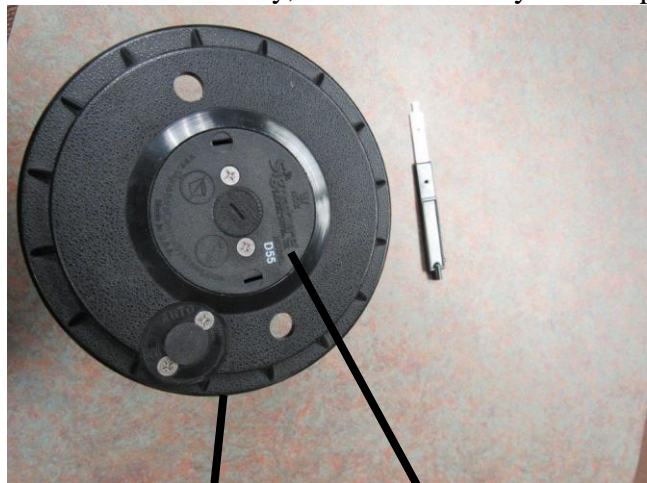
Photos of Rotor Body, Internal assembly and Snap Ring Tool.
