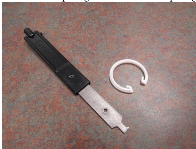
Photo of Snap Ring Tool and white Snap Ring.
