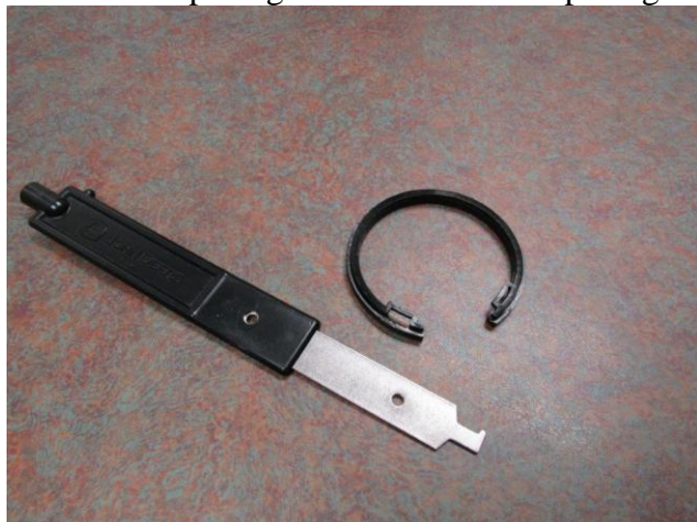
Photo of Snap Ring Tool and black Snap Ring.
