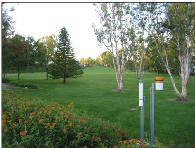
In foreground, ET gauge (left) and tipping rain bucket (right) at Casta del Sol Homeowners Association - Mission Viejo, California
