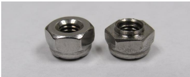
Old nut New Nut (Machined Side)
