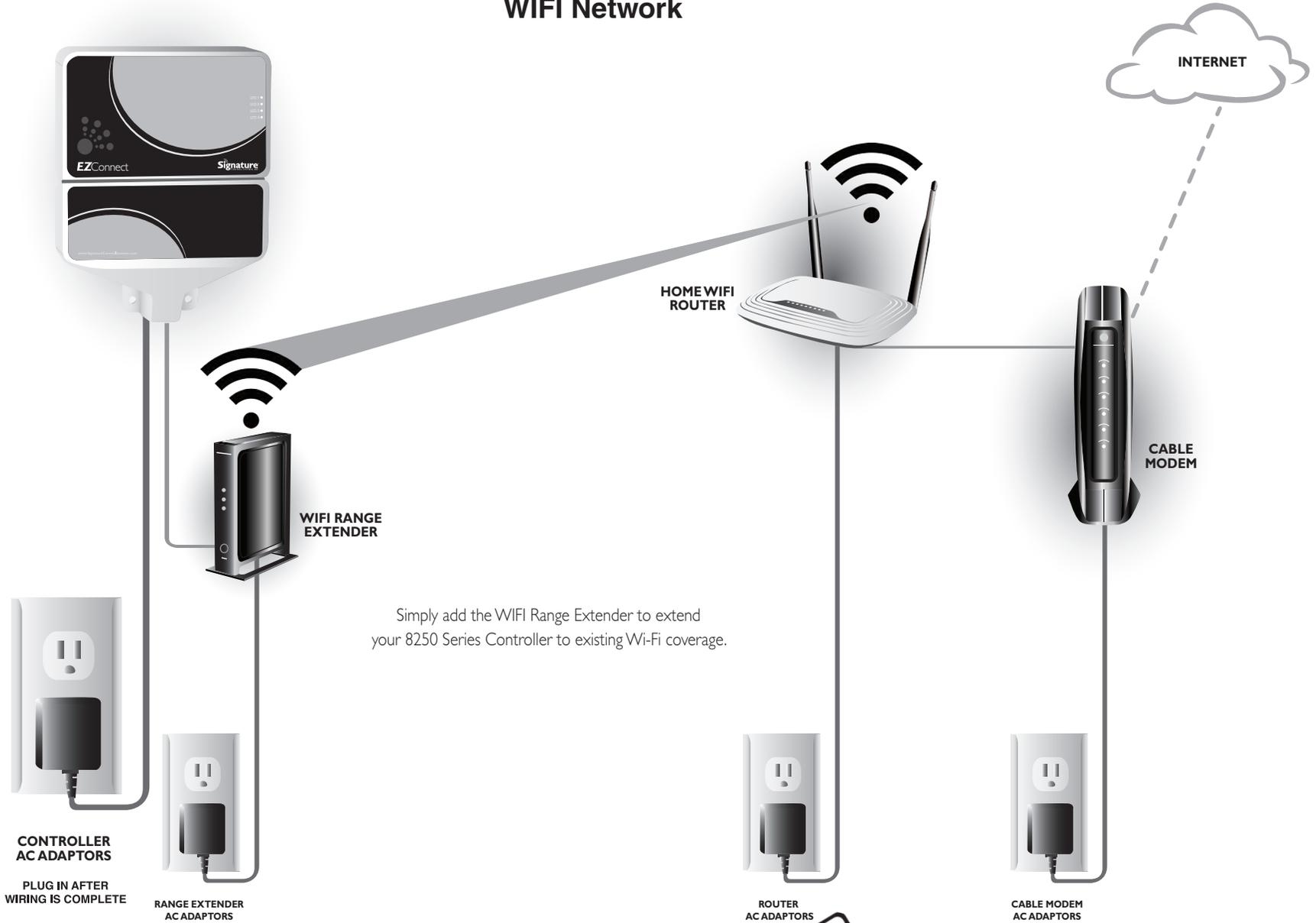
Simply add the WiFi Range Extender to extend your 8250 Series Controller to existing Wi-Fi coverage.
