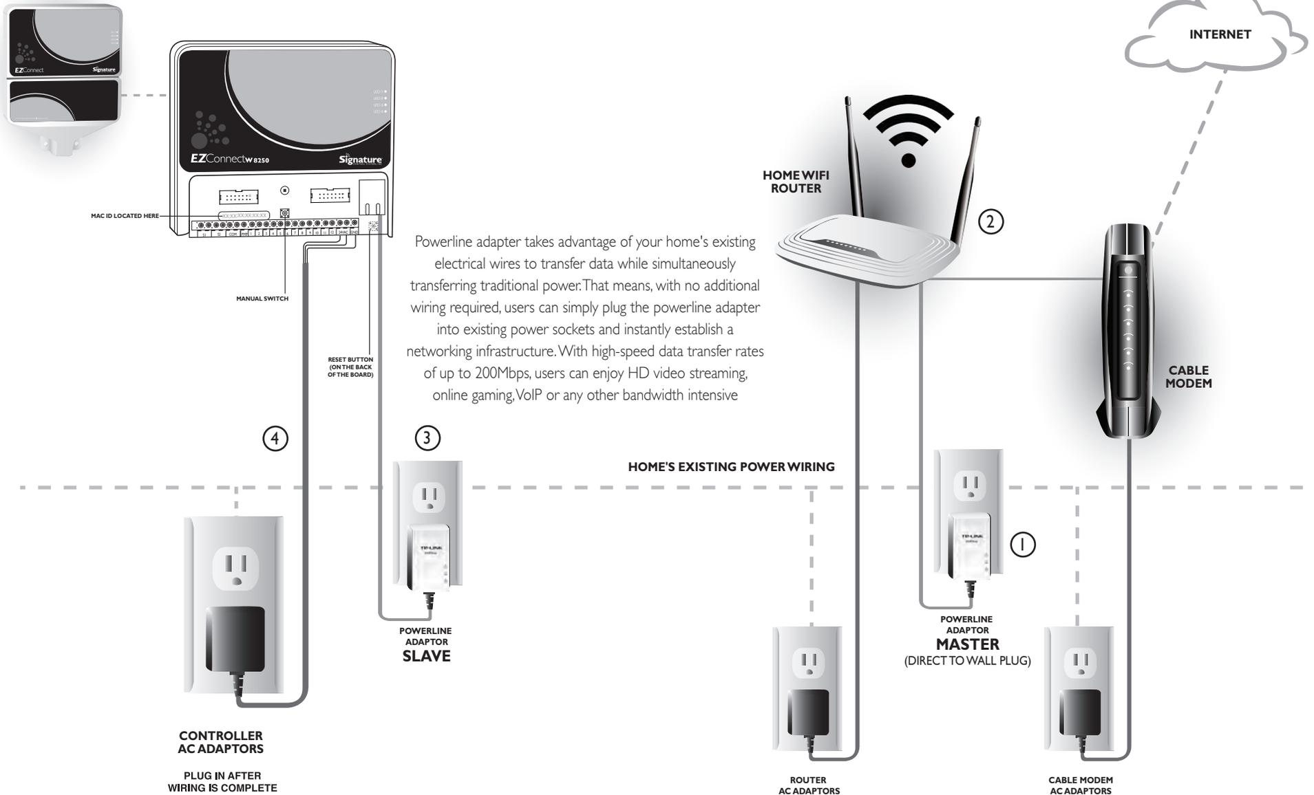
Powerline adapter takes advantage of your home's existing electrical wires to transfer data while simultaneously transferring traditional power. That means, with no additional wiring required, users can simply plug the powerline adapter into existing power sockets and instantly establish a networking infrastructure. With high-speed data transfer rates of up to 200Mbps, users can enjoy HD video streaming, online gaming, VoIP or any other bandwidth intensive
